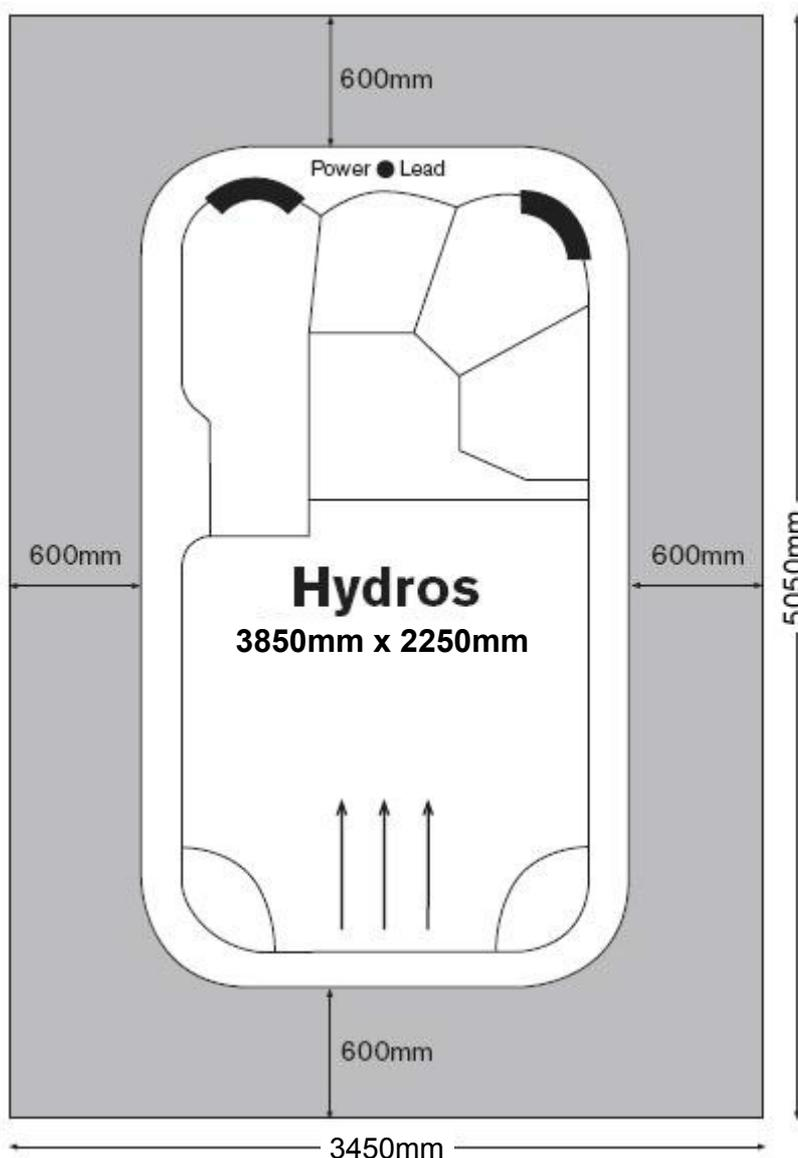
In Decking: If you are sinking your pool and decking around it please remember to build the decking to allow access to the electrical compartment and all components. Please ensure the electrical compartment has some ventilation for correct functioning. If decking up to/around pool, we would recommend decking after installation.
