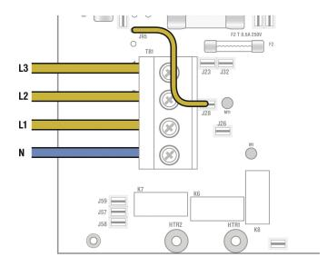
Note: J57, J58 and J59 are electrically identical. The blue wire may be attached to either of these terminals before removal.
