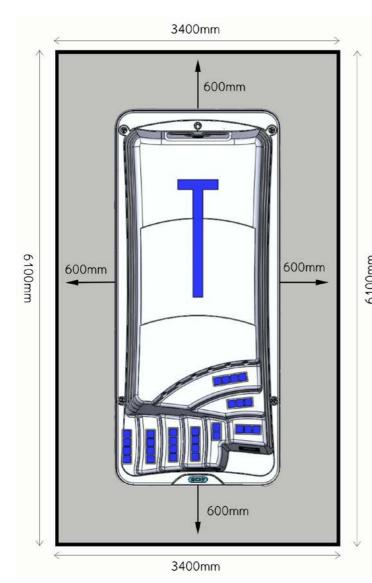
When digging your hole please allow 600mm gap at the control panel end and 150mm gap around the other three sides of the pool. This gap will also allow for airflow and tolerance of natural movement from water volume when filled. Dig the hole and lay a 6" (16cm) reinforced concrete base with a soak away underneath and ensure the pit has retaining walls of sufficient structural strength (back filling is not recommended).
