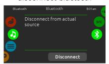
If a device with Bluetooth technology is connected to the in.stream 2, you can disconnect it by pressing the Disconnect key at the bottom of the screen
