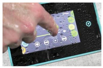
The Gecko in.k1001 capacitive touch screen display keypad will operate under wet and rainy conditions.
