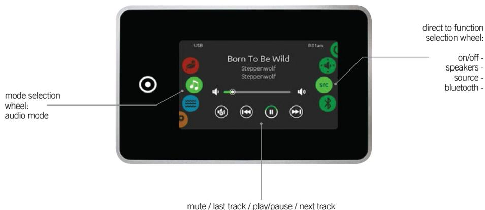
To select the audio mode, slide the left wheel up or down until the audio icon menu is highlighted in the middle.
