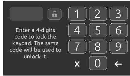
When the user wants to lock the keypad he is asked to select a 4-digit code. The same code will be needed to unlock the keypad.
